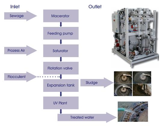
All sewage needs to be collected in one ship's holding tank. Depending on the calculated load and number of persons the tank must have a sufficient size as the working volume between high level and stop plant is one important issue for the HL Cont PLUS.
